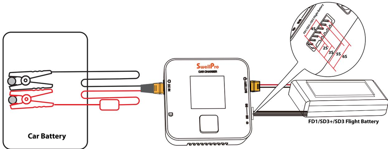
For FD1/SD3+/SD3 flight battery: Plug in the yellow XT60 connector to the “BATTERY” port of the charger. Plug in the balance cable to the “2S – 6S” port of the charger. **Note: the balance cable should align to the bottom pin of the port.**
