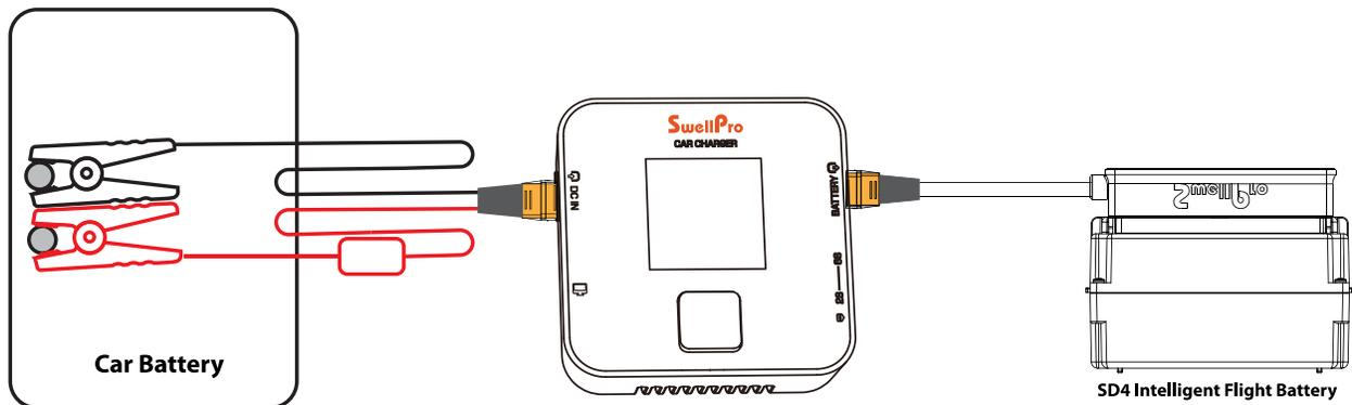
**For SD4 intelligent flight battery:** Use the in-the-box SD4 charging cable. Connect the SD4 intelligent flight battery on one end of the charging cable. Plug in the yellow XT60 connector to the “BATTERY” port of the charger.
