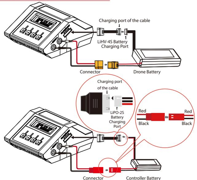
1. Before charging, check and make sure the terminals and wires of the battery pack are not damaged.
